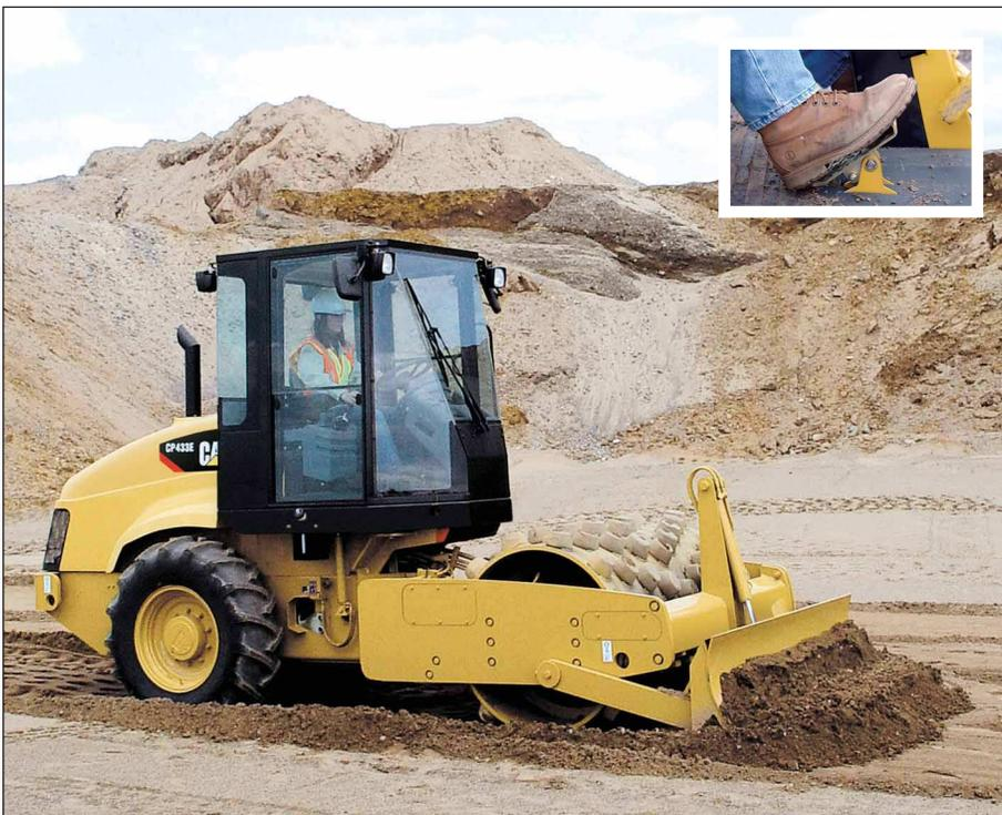
**Expands machine versatility and utilization** for use in material knockdown, site leveling, trench backfilling and light dozing applications.
