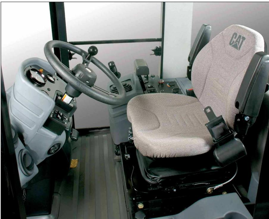
**Steering console and operational gauges** on the CS433E and CP433E are infinitely adjustable within the tilt range to the desired position of the operator. Entire console tilts for simple entrance and exit.
