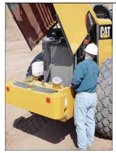
The fiberglass hood tilts forward for good access to the engine and cooling system. Daily service points are accessible from ground level and are grouped on one side of the machine.
