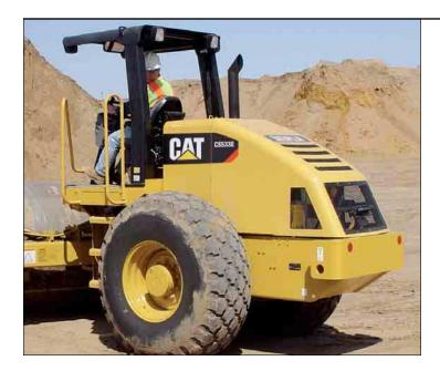
**Visibility.** The visibility to the tire edges and rear of machine is exceptional. The sloped hood allows the operator to see obstacles measuring 1 meter high located 1 meter to the rear of the machine. Excellent visibility increases productivity when working near obstructions or maneuvering around the job site.
