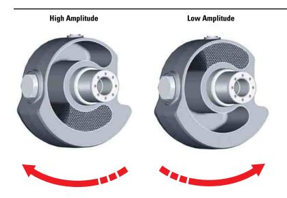
**Amplitude selection.** Positive amplitude selection is accomplished when the steel shot is repositioned inside the hollow eccentric weight. Direction of weight shaft rotation determines amplitude level.
