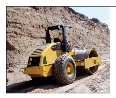
**Propel pump system.** Two propel pump system has dedicated pumps to drive the heavy-duty, high-torque rear wheel and drum motors independently. Should the drum or wheels begin to spin, the non-spinning motor still receives hydraulic flow, allowing continuous tractive effort especially useful in loose underfoot conditions.
