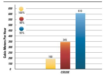
% Compaction of Standard Proctor 150 mm Crushed Limestone Base Results are similar for padfoot drums. Results may vary for different applications.
