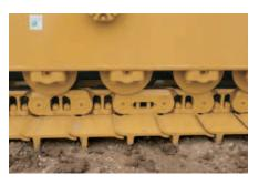
**Roller Design.** The SystemOne<sup>TM</sup> roller has a taller flange to improve track guiding, especially in side-sloping applications. Advanced features and reduced piece parts enhance the rollers which help eliminate any flexing in the collars and avoid oil loss. The roller is maintenance-free and serviced as a group only. To achieve total balanced wear, carrier rollers with increased wear life are also used.
