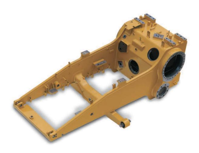
**Frame and Castings.** The D6R III frame is built to absorb high impact shock loads and twisting forces. The frame has a reinforced saddle and a welded front cross-member that add strength to the frame to better handle lateral and twisting forces. Steel castings augment the strength of the main case.
