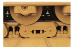
**Master Link.** A unique feature of the System One Undercarriage is that, unlike traditional undercarriage, a master style link is not required. This improves track reliability and durability. The unique straight link design allows the track to be taken apart at any joint by using the proper Caterpillar tooling to press the link on or off. A clamp-style master link is available but not recommended for high impact conditions or machines using wide shoes in these types of applications.
