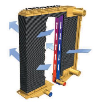
Advanced Modular Cooling System (AMOCS). Using a two pass system, the AMOCS radiator provides more efficient heat exchange and improved cooling capacity over the D6R Series II. The coolant is routed from a sectioned bottom tank up the front side, over the top of the core and down the engine side of the core to the bottom tank. This flow pattern allows the coolant to pass through the radiator twice for better cooling.
