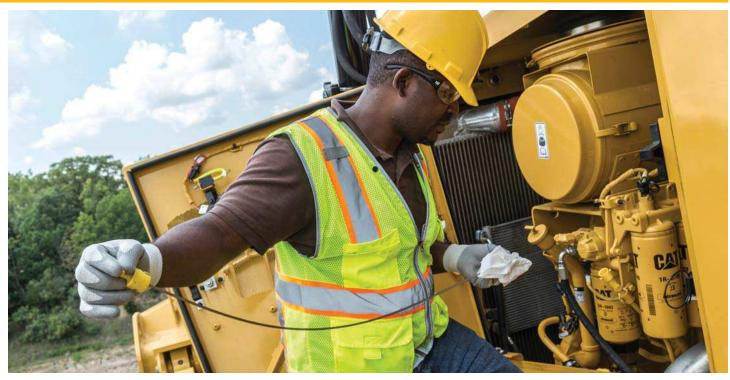
Like all Cat dozers, the D8R is designed with features like wide engine panel access doors to minimize maintenance and repair time. You can also outfit your dozer with these optional service features to make maintenance even easier so you can get back to work faster:
