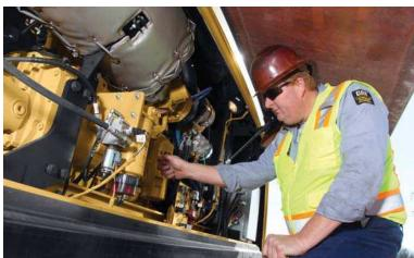
To ease serviceability on the MH3049, all primary service points are conveniently located under a single access service panel on the right side of the machine or beneath the top engine access panel. Easily locate components with the engine and cooling system's longitudinal layout. Both panels are hinged with gas struts, ensuring that one technician can easily access all maintenance points.
