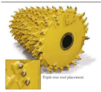
**Universal Rotor.** Designed primarily for use in asphalt reclamation.
