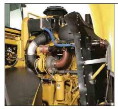
Large one-piece fiberglass hood tilts forward for exceptional access to the engine and cooling package. Daily service points are accessible from ground level and are grouped on one side of the engine. Lower side panels open wide for even greater access.
