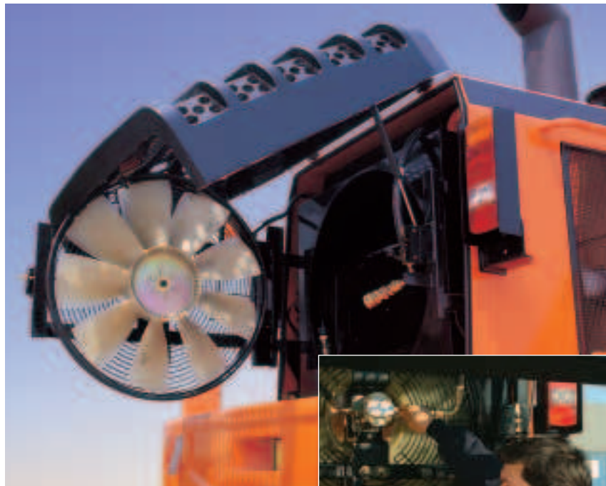
The radiator cooling circuits, as with the engine oil, can be remotely drained with ease, therefore safely respecting the environment.
