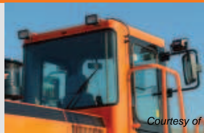
Powerful front and rear working lights ensure an excellent view of the work area day or night.
