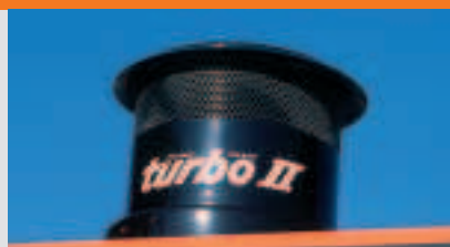
A large capacity air cleaner, combined with a Turbo II pre-cleaner, allows reduction of the cleaning or the servicing of the main cartridge.
