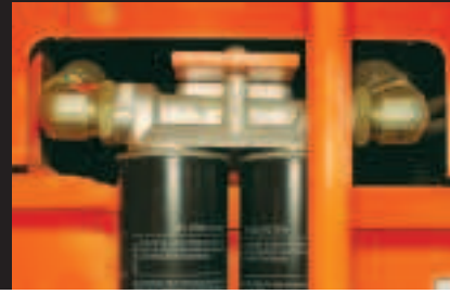
The hydraulic return line is filtered to within 10 microns.
