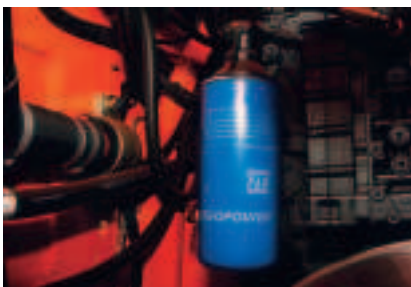
The transmission filter(s) are within easy reach and like the rest of the machine's service components can be checked from ground level.
