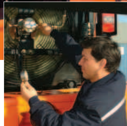
The cooler fan swings clear for ease of cleaning. The Daewoo technical service department can, under specific circumstances, regulate the cooling fan, allowing optimal cooling – to suit extreme conditions.
