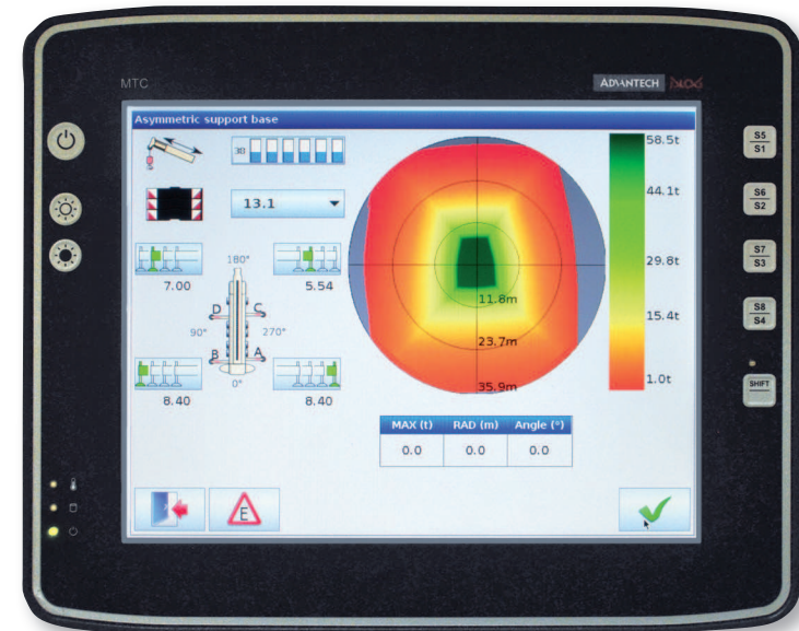
On-board simulation with IC-1 Plus control system
