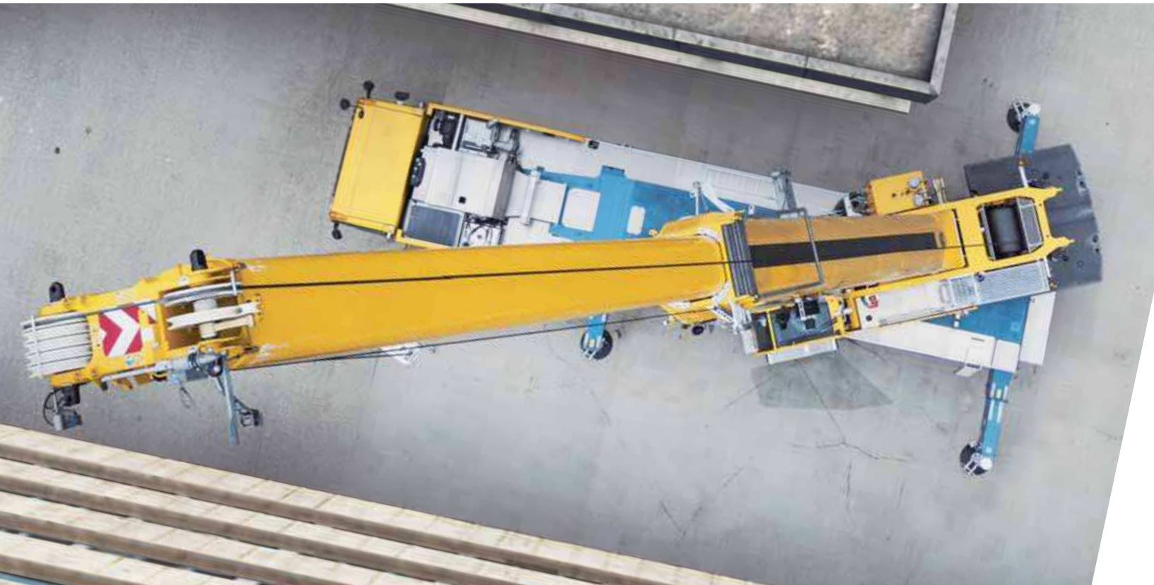
Asymmetric outrigger setup for confined spaces
