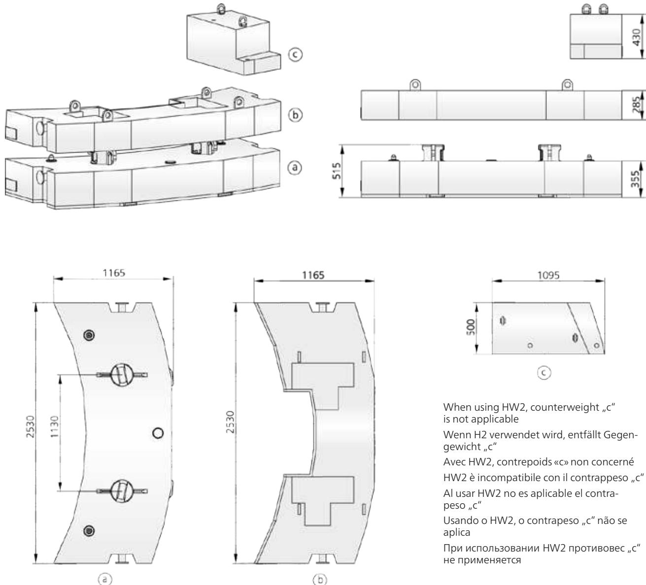
When using HW2, counterweight „c“ is not applicable
