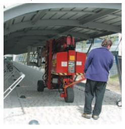
Narrow areas and doorways were easy to negotiate due to the Denka's compact size of 0.89m wide x 2.1m high. The Denka DL 22N weighs only 2,350kg which made it suitable for the Velodrome's lightweight
