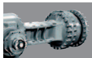
Hydraulic differential lock For automatic (depending on transmission torque) or manual differential lock.
