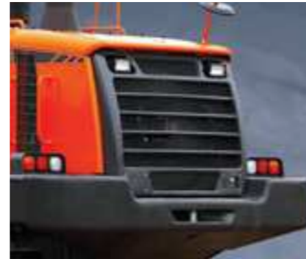
Radiator Grill (Steel structure)
