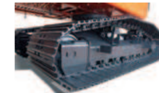
High track (on DX160LC-3) Ideal in forestry, recycling and demolition due to its higher ground clearance (15 cm).
