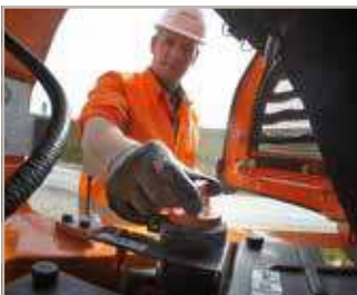
Battery cut-off switch
