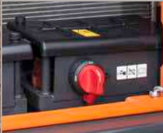
Battery cut-off switch
