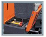
Battery Box The battery is located on the side of the machine and can be reached easily by opening one key operated panel.
