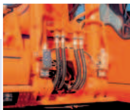
Boom and arm hose rupture protection valve
