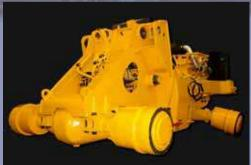
The front frame with high mount boom cylinder pivots increased lifting ability to the top without sacrificing digging ability. The rear frame features trunion rear axle
