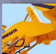
Z-Bar linkage transfers maximu force to the bucket to pry out h
