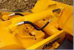
Integral solid boom arms combine a large cross tube and castings to provide a strong structure, which gives excellent stress distribution for the bucket, yet provide extra stiffness during bucket corner loading.
