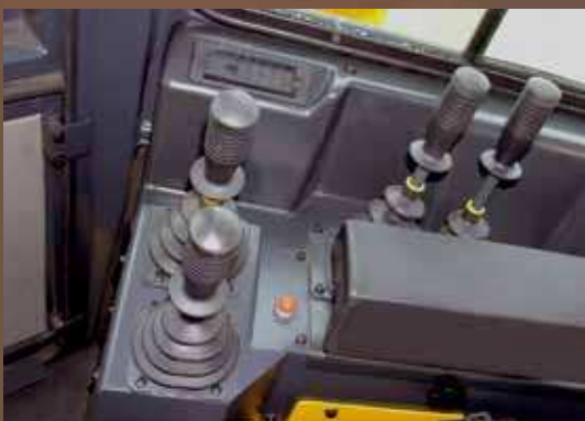
The two front levers control winches of the pipelaying equipment while the side levers actuate the counterweights that maintain the proper stability of the machine.
