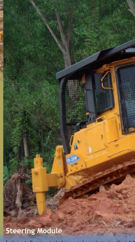
Exclusive to Dressta, standard two-speed geared steering allows full power turns for full load retention, lowers sprocket and track bushing wear, increases ripping operation performance and allows greater directional control in both slope work and side cutting.
