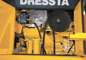
The Tier 3 approved Cummins QSK19 engine with state-of-the-art electronic controls and modular common-rail fuel system ensures clean, efficient performance, minimum maintenance and superior uptime. Multi-unit modular cooling package with hydraulically driven, variable speed fan improves cooling efficiency.
