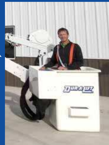
GROUND ACCESS FROM BASKET
