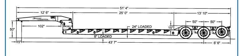
Capacity: 110,000 lbs. Trailer Weight: 21,225 lbs. Deck Width: 8 ft. 6 in. Length: 25 ft. Height: 24 in. (Loaded) 80.000 lb. Minimum Yield Steel Mainframe **Pierced Crossmembers** Front Flip Ramps, Stressed for 4th Flip
