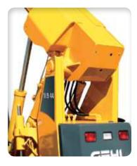
ADDED STRENGTH, durability and longevity are achieved with the double-wall rear tower and robust, heavy-duty boom nose.
