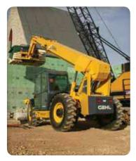
**STANDARD SAHR** (springapplied, hydraulic-released) parking brake is located on the front axle. It applies automatically when the engine is shut off, or by simply pressing a rocker switch.
