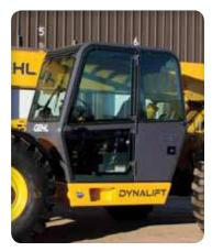
**CAB OPTIONS** in an open canopy for mild climates and rental applications or enclosed with heater and defroster. Air-conditioning is optional on the enclosed cab models.
