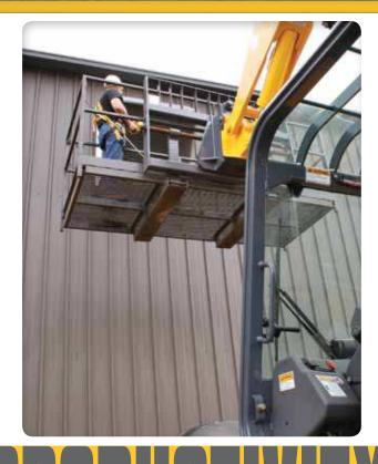
PERSONNEL WORK PLATFORM (PWP) SYSTEM The optional Gehl PWP System allows the safe and efficient use of an ANSI/ITSDF B56.6 compliant work platform.
