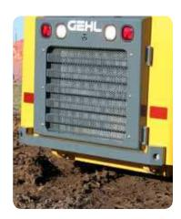
optional and boost the rated load capacity to 2,110 lbs. (957 kg) on the R190, 2,370 lbs. (1075 kg) on the R220, and an impressive 2,780 lbs. (1261 kg) on the R260.
