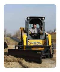
ACCELERATE RAPIDLY with maintenance-free, radial-piston drive motors with high start-up torque and maximum ground speeds up to 12.5 mph<sup>1</sup> (20 km/hr).
