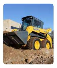
**STABLE RIDE** is achieved with a longer wheelbase and low center-of-gravity. The HydraGlide<sup>TM</sup> ride control option provides smoother operation over uneven surfaces.
