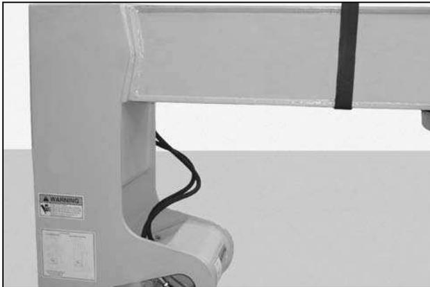
Slide the inner boom section into the intermediate boom up to the balance point, then reposition the lifting strap and slide the inner boom in until there is approximately 12 inches (300 mm) of the inner boom sticking out of the intermediate boom.
