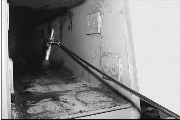
With the inner boom section removed, apply grease to the inside bottom and top surfaces of the intermediate boom section where the pads of the inner boom will contact when assembled. Use a brush attached to a rod or pole (as shown) to reach inside the boom.
