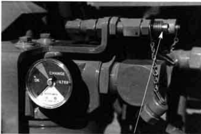
TAKE HYDRAULIC OIL SAMPLE FROM THIS PORT
