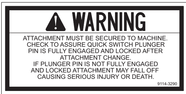
Located on left side of boom head P/N 9114-3290
