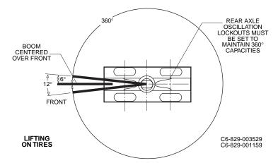
BOLD LINES DETERMINE THE LIMITING POSITION OF ANY LOAD FOR OPERATION WITHIN WORKING AREAS INDICATED
