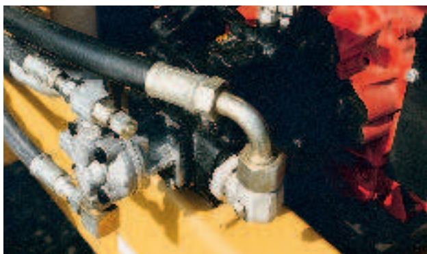
Piggy back gear pump provides priority flow for steering.
