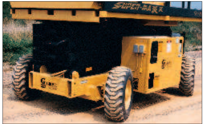
Optional four-wheel steering makes it easy to maneuver close to walls and through congested job sites.
