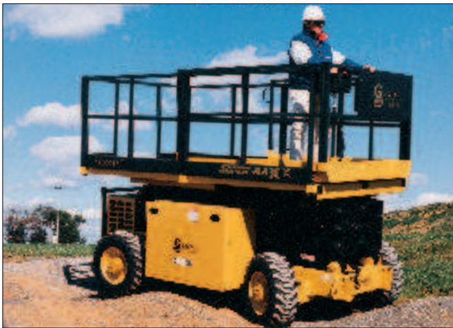
SUPER-MAXX Series XT versions offer standard four-wheel drive.
