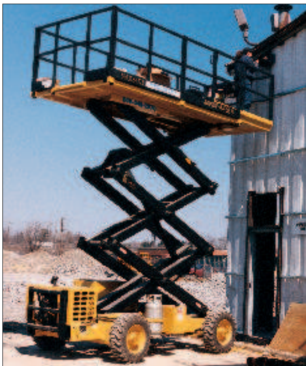
Large standard deck offers 71.9 sq. ft. (6.7 m 2 ) of area.
