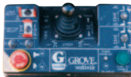
Convenient removable control box features patented enable button.
