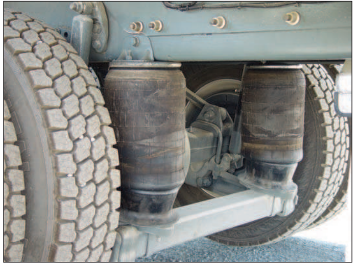
Spring front suspension w/air ride rear suspension provides a comfortable ride at 65 m.p.h. (105 Km/h)
