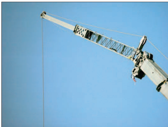
Max. tip height of 154 ft. (47.0 m) w/ 45 ft. (13.7 m) tele. extension
