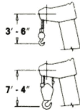
DIMENSIONS ARE FOR LARGEST GROVE FURNISHED HOOK BLOCK AND HEADACHE BALL, WITH ANTI-TWO BLOCK ACTIVATED.
