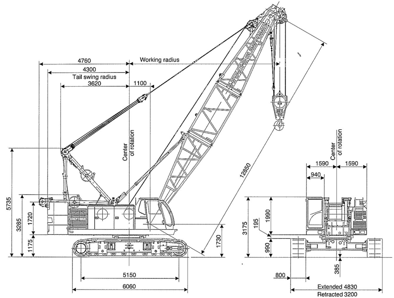
Notes: The above general arrangement is under liftcrane application with 12.85m basic boom, optional 80t hook block and optional 3rd drum.
