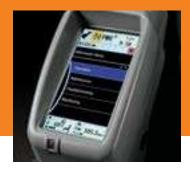
Multi-language LCD monitor and rotary dial provide intuitive access to machine info and functions. Just turn and tap to select work modes, monitor maintenance intervals, check diagnostic codes and set cab temperature. Control oil flow and toggle between dig and thumb modes with a programmable thumbattachment mode.
