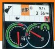
■ Easy-to-navigate LCD monitor issues scheduled maintenance alerts and diagnostic information. Additionally, the hydraulic temperature gauge on the monitor screen helps prevent downtime.
