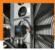
A reversing fan back-blows cooler cores to reduce debris buildup and increase uptime.
