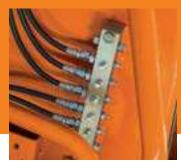
Centralized lube banks place zerks within easy reach, making greasing less messy and timeconsuming.
