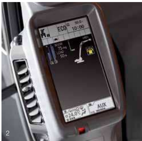
Swing angle alarm and HRD overload warning system
