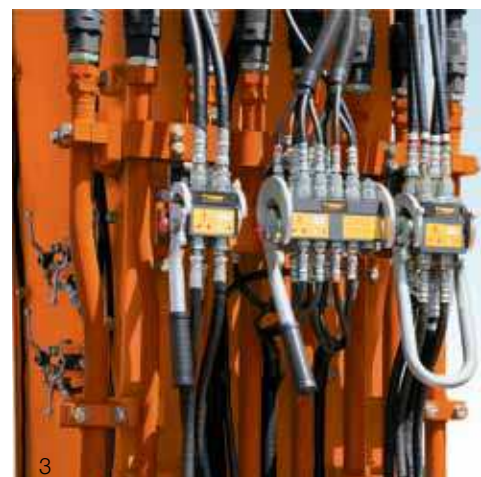
3 Lever type quick couplers
