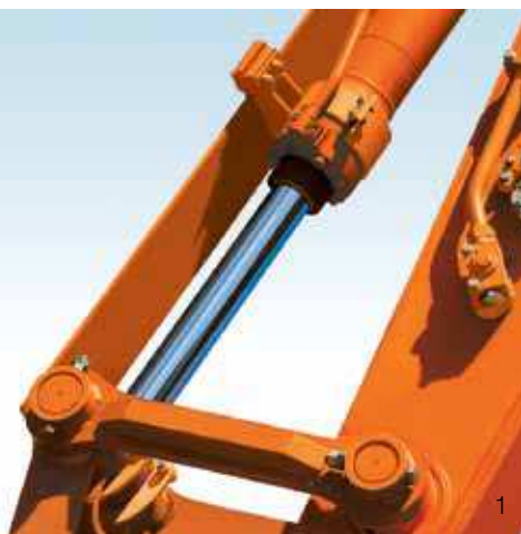
Tilt cylinder guard
