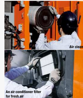
An air conditioner filter for fresh air
