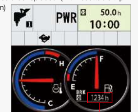
Breaker hour meter
