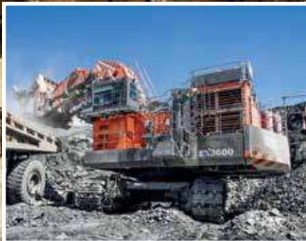
EX ultra-large excavators
