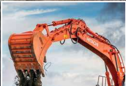
Reinforced boom and front attachment.
