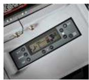
Automatic, high-velocity bi-level climate-control system with automotive-style adjustable louvers help keep the glass clear and the cab comfortable.
