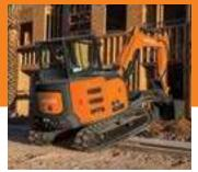
Choose the tracks that are best for the way you work. The rubber tracks traverse virtually any terrain, including paved surfaces. Also available are steel tracks and steel tracks with rubber pads. The optional rubber grousers combine workanywhere flexibility with steeltrack serviceability.
