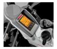
Enhanced monitor provides vital operating info at a glance and fingertip control of several functions, including autoshutdown, power/economy modes and auto exhaust filter cleaning. Plus, two trip meters let you track engine oil and hydraulic oil changes, or jobsite hours.
