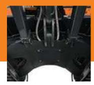
Heavy-duty X-frame provides a solid, stable platform that resists material and dirt build-up.
