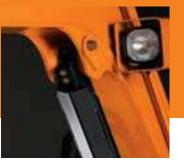
Heavy-duty shields deflect material and impacts, protecting the boom/blade cylinders and drive motors.
