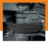
Single-pin swing-post increases boom stiffness, enhancing the structural integrity of the digging components. Wear-resistant hoses are routed for protection and Cordura®-wrapped where exposed.
