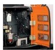
Hinged door provides wideopen access to the side-by-side oil cooler and radiator for easier core cleanout.
