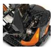
Operator station tilts forward 50 degrees, simplifying access to the swing motor, hydraulic control valve, engine starter motor and alternator.
