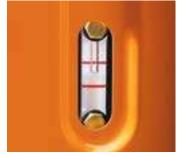
Hydraulic fluid sight gauge and see-through coolant reservoir let you quickly check levels at a glance.
