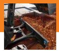
Although not a replacement for a grading tractor, standard backfill blades let these excavators fill in quite capably. An optional all-hydraulic blade angles 25 degrees, left or right, for even more efficient grading and backfilling.
