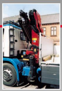
◄ HMF-loaders are developed with great importance attached to reduced chassis space requirements, in order to obtain as much space as possible for the body building. The HMF 1560 Series without extra valves thus has a chassis space requirement of only 830 mm.
