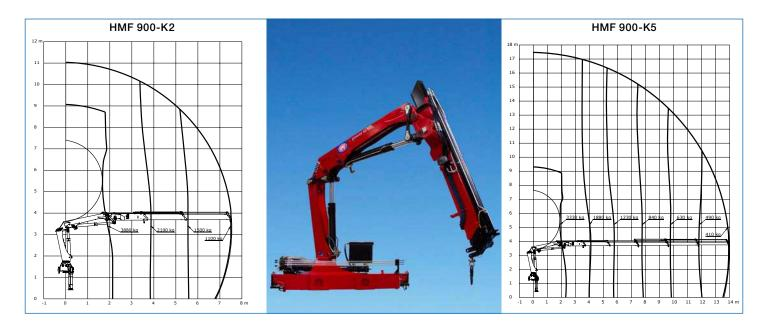
The HMF 900-K model with dual Power Plus link arm system and manual ground control or stand-up controls and fixed flow pump.
