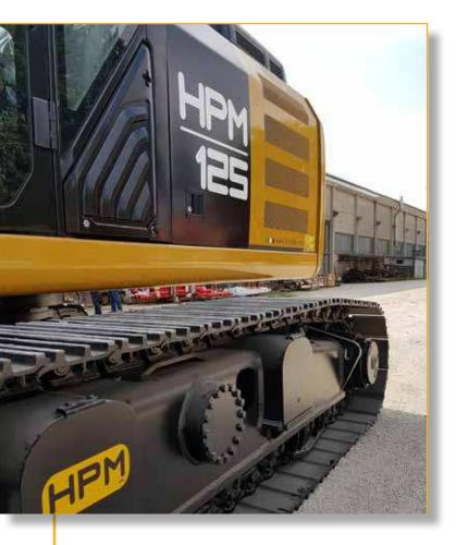
The HPM125 is mounted on a CAT 323FN Tier IV base, this reliable drilling rig result extremely friendly and efficient operation and maintenance.
