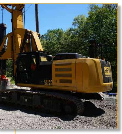
The HPM200 is mounted on a CAT 330F Tier IV base, this reliable drilling rig result extremely friendly and efficient operation and maintenance.
