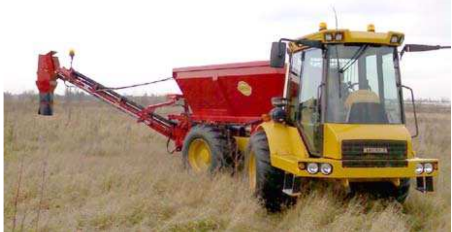
Here the previous model, 912C Series 2 with MultiChassis, mounted with a Bredal K65 sand distributor.
