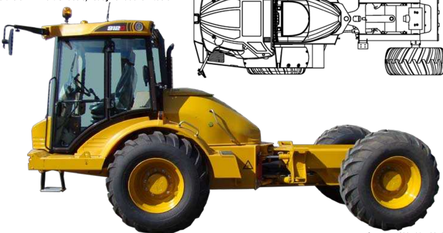
The MultiChassis seen from above. Here the 912D MultiChassis, ready for add-on-tools.
