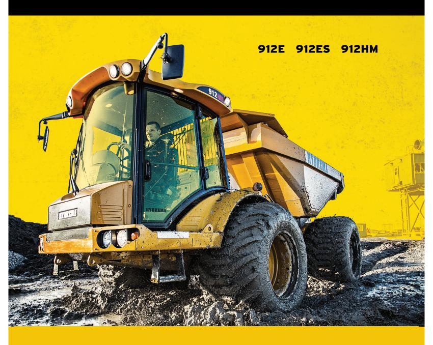
A unique combination of articulated center pivot, wide wheels and high ground clearance. For high mobility and low ground pressure.
