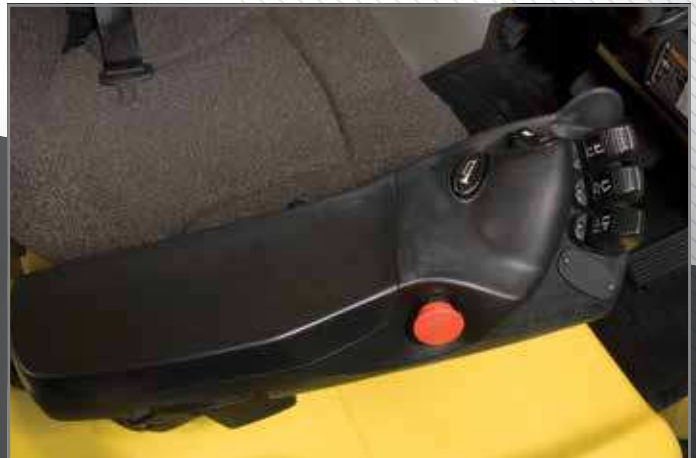
Electro-hydraulic controls with TouchPoint mini-levers
