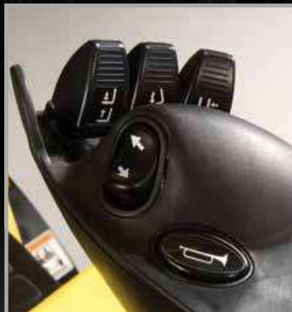
TouchPoint mini-levers with seatside direction control
