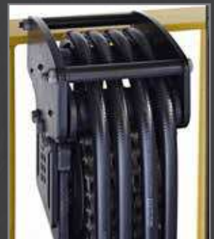
Free lift hose protection reduces likelihood of damage.
