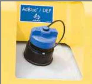
Diesel Exhaust Fluid (DEF) tank.
