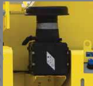
Tier 4 Final integrated pre-cleaner and air filter.
